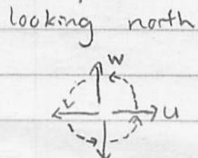
If we adopt the hydrostatic approximation then  $-\frac{1}{\rho} \frac{\partial P}{\partial z} = -g$  and  $\frac{dw}{dt} = 0$ . This means the Coriolis term in the  $w$  equation must be neglected; otherwise, the term would cause  $\frac{dw}{dt} \neq 0$ .
